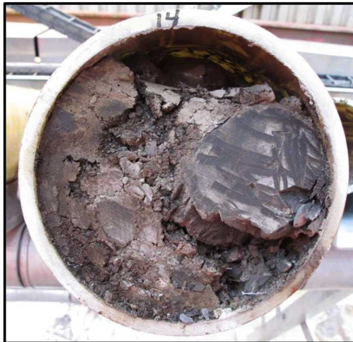
Figure 2—Core photo of core 2 at xx14m. Considerable apparent damage can be observed in the core.
